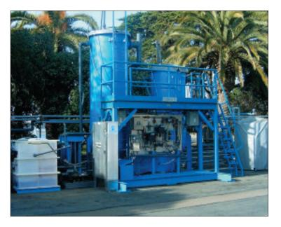
Mobile pilot units are available to demonstrate the DynaSand D2® System's ability to process site-specific source waters. The pilot units are equipped with full monitoring and reporting capabilities and demonstrate the ease of operation of the DynaSand D2® Advanced Filtration System.
