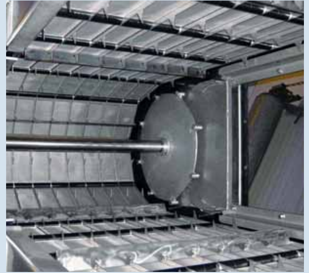
This grid drive sprocket design is unique to the Hydro-Flo. No chains are required, making it simple to operate and maintain while greatly reducing wear and horsepower requirements.
