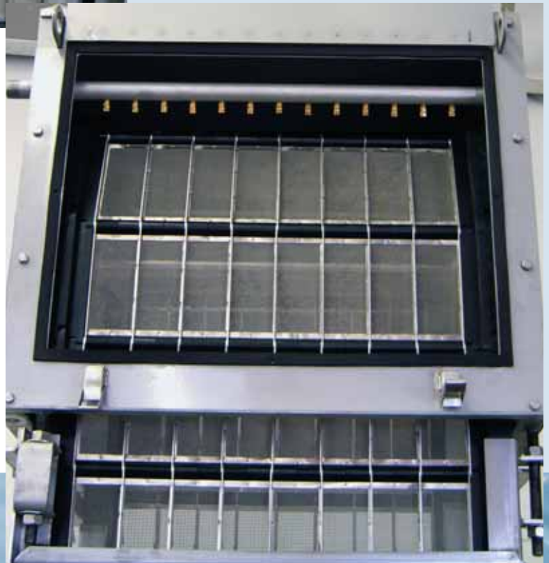
Huge access panels provide ample access for inspection and maintenance of grid and spray header.
