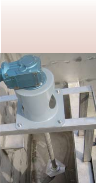
MRI MANUFACTURES VERTICAL TURBINES (SHOWN), HORIZONTAL PADDLE WHEELS AND HYDRAULIC BAFFLES TO MIX AND MATCH.
