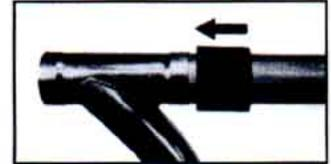
**2** Join tubing and fitting together. Center Shrink Sleeve over joint.
